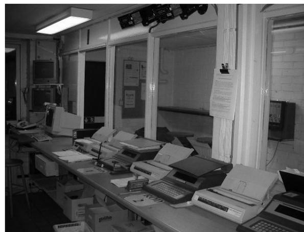
Figure 2. Above the desk, near the ceiling are three scales (black “boxes”) used for monitoring grain transportation processes. On the desk lie printers (connected to the scales) and piles of documents.
